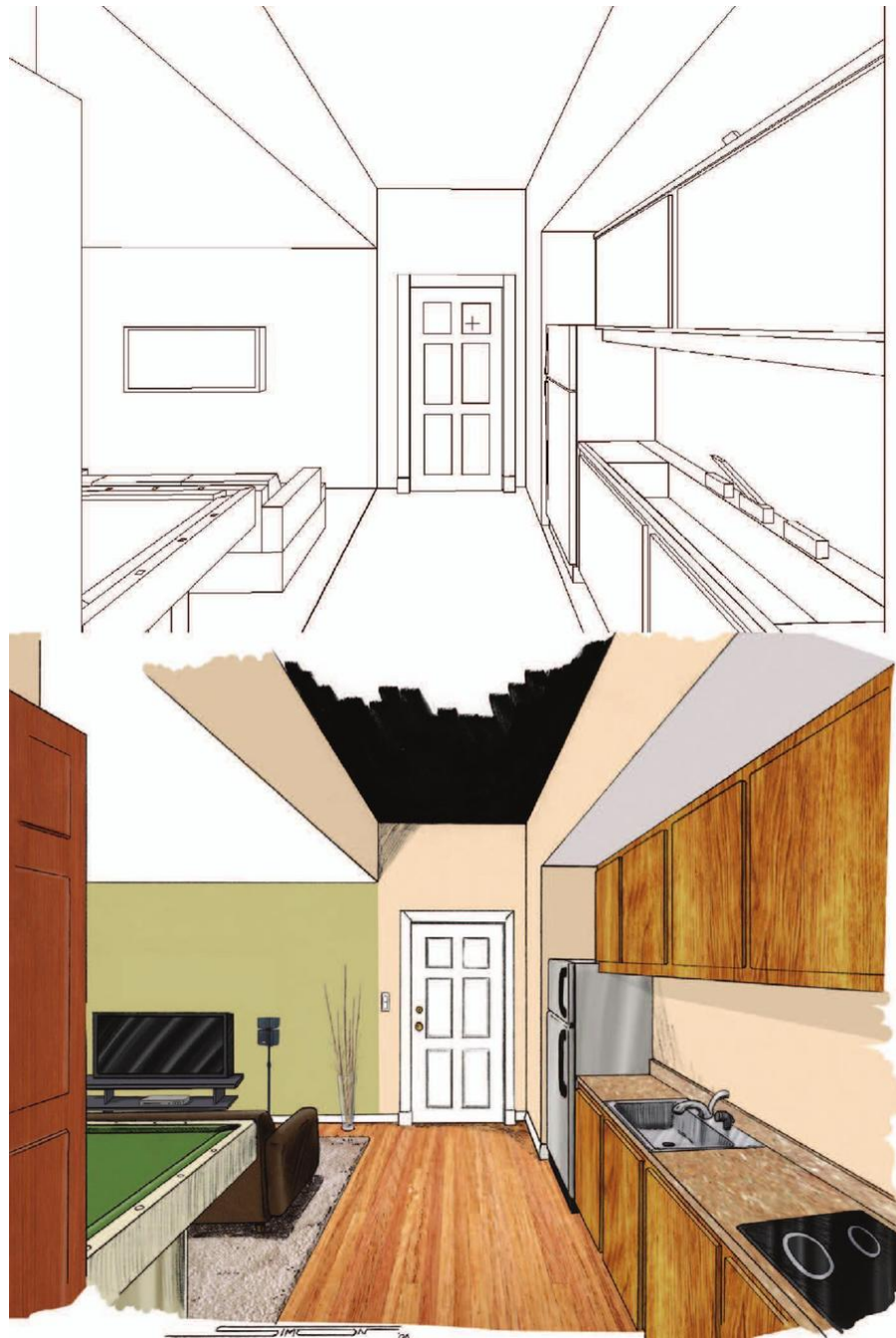
Figure 8.7 The top image shows hidden-line removal from a 3D program. The bottom image shows the final rendering. The final lines were drawn by hand and colors and textures were painted in using Photoshop.
